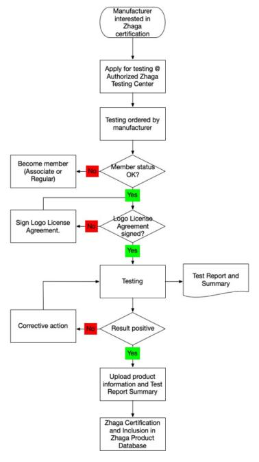
Figure 4-1: Process for Zhaga certification of a product.
