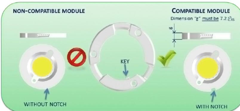
In the “Locking Ring” configuration the module shall fulfil the following characteristics:
