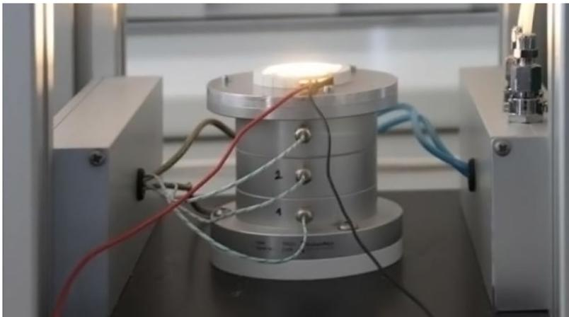
**The Test procedure for measuring  $P_{th,rear}$**
